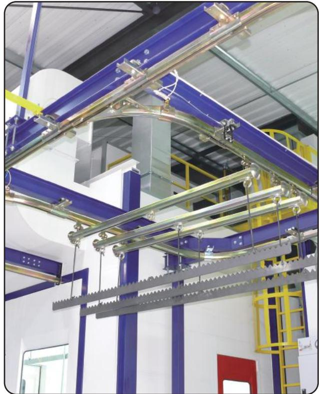
Power & free conveyor is highly automatic and integrative, which can stop individual loads without stopping the entire production line. The main conveyor is moving continuously, but another loading conveyor just move step by step, the output capacity can be very big if the main conveyor speed is fast, no need to enlarge the oven size. So it takes smaller space than the common tunnel oven design.
